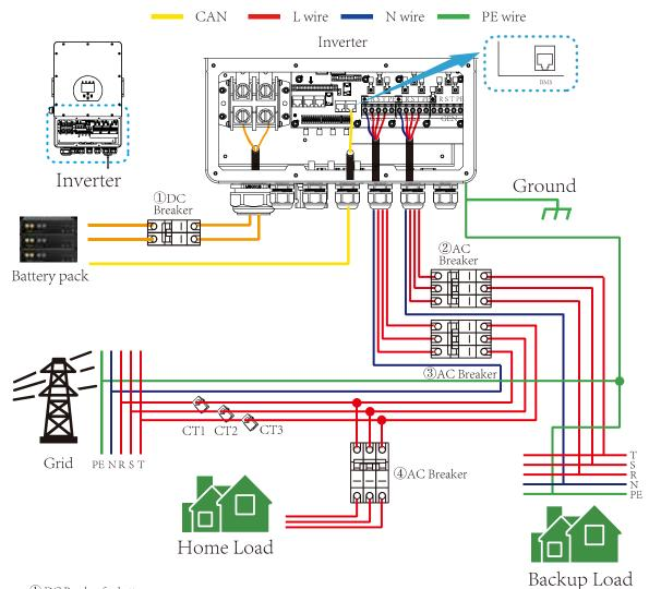
① DC Breaker for battery SUN 8K-SG: 250A DC breaker SUN 10K-SG:300A DC breaker SUN 12K-SG:300A DC breaker
